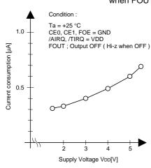
(3-2) Current consumption when non-accessed (ii) when FOUT=32.768 kHz
